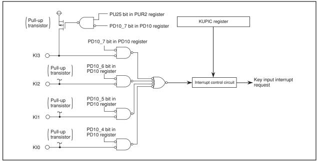
Figure 9.14 Key Input Interrupt Block Diagram
